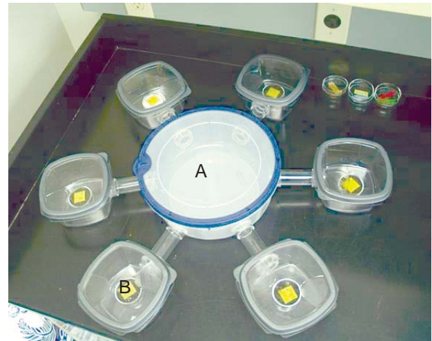
Fig. 1 Six-armed experimental arena used for all experiments in the study. A 60 × 15 mm glass Petri dish containing the treatments (e.g. growing medium) was placed into the designated sample compartments (B). A 2.5 × 2.5-cm yellow sticky card was placed onto the surface of each treatment. Adult fungus gnats, Bradysia sp. nr. coprophila , obtained from a laboratory colony, were collected in a plastic vial and then placed into the central compartment (A). The number of adult fungus gnats captured on the yellow sticky cards and on the floor in the sample compartments (B) was used to measure the attractiveness of each treatment.
